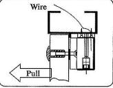
Close and pull the door to test holding force, Extra washers can be added to adjust angle between door leaf and Armature plate.
