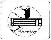
Confivm the holding Fovg and tighten the proof Screws.
