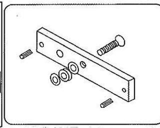
awcoding to the picture add the washers on the Armature.
