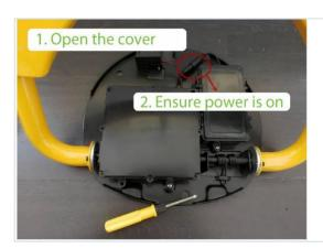
Open the cover, press the botton for more than 3 seconds. The code is deleted after one ticking
