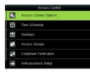
Access Control Options: Including Door Lock Delay, Door Sensor Delay, Door Sensor Type, NC / NO Time Period etc. Time Schedule: Schedule Doors' opening time, 50 time zones are available to define.
