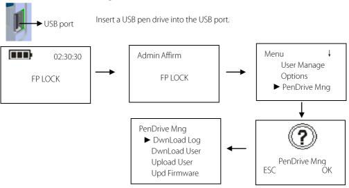
Note: If you want to do USB Pen Drive management, the band switch must be set at the middle position. Otherwise the fingerprint lock cannot detect the U disk.
