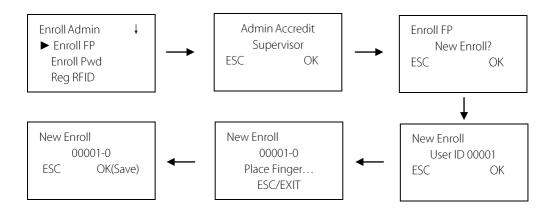
The system will prompt to save the enrollment information after the enrollment is successful. If the enrollment fails, the system will prompt to re-enroll fingerprint. The system returns to the "New Enroll" interface upon successful enrollment. You can continue or exit the fingerprint enrollment at that time.
