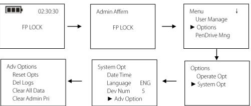
The advanced options include Reset Options, Delete Logs, Clear All Data and Clear Administrator Privilege. Press 2/3 to select the desired option, and then press MENU to enter the menu. Select the items and press MENU to execute the corresponding operation. The screen will return to "Advanced options" menu. If you press 1 (ESC) and quit, it will return to the advanced option menu without any operation.
